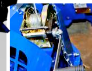
Conveyor lifting /lowering winch
