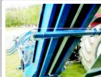
Discharge conveyor (4m): two stage telescope with automatic hydraulic belt straining. Continuous speed control of the conveyor belt.
