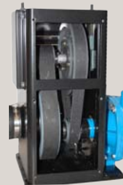
Incoming PTO speed is increased through a series of sheaves
