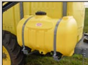
Fresh Water Rinse System
